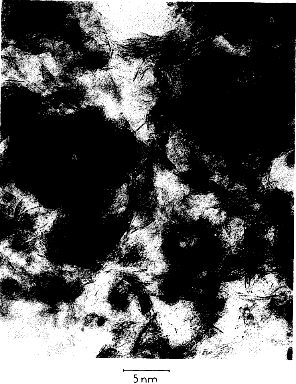
FIG. 5. Additional TEM micrograph of a delaminated laponite showing the distribution of aggregates containing about 4 to 8 unit layers held together by face-to-face connections. Some poorly crystallized alumina is also present (A).
